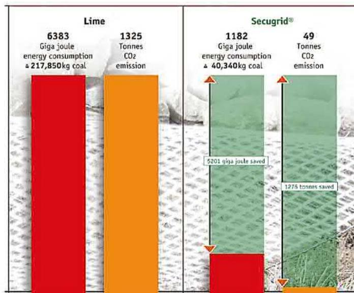
**Figure 4: Environmental savings based on accumulated energy and CO<sub>2</sub> consumption: Lime vs geogrid stabilisation**
