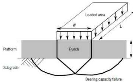
**Figure 12: Bearing resistance of a platform on soft soil (BRE470, 2004)**
