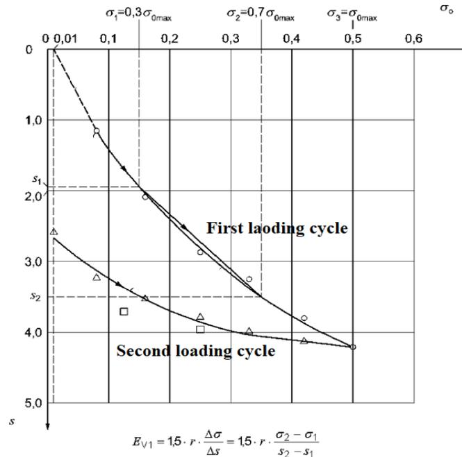
**Figure 8: Load-settlement curve and fitting curves for the first and second loading cycles, and example calculations for  $E_{v1}$  (DIN 18134, 2012)**
