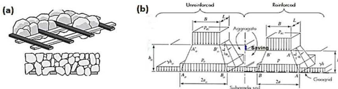
**Figure 3: Aggregate-geogrid interlocking and confinement (a) and thickness reduction as a result of geogrid reinforcement and stabilisation (b)**
