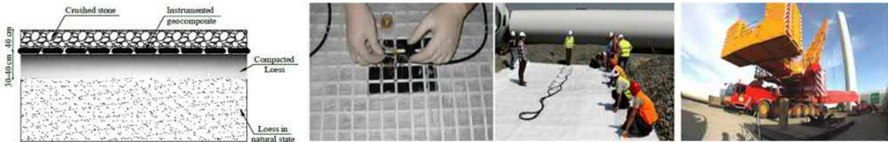
Figure 15: Combigrid reinforced working platform field trial and measurement (Batali et al., 2014a)
