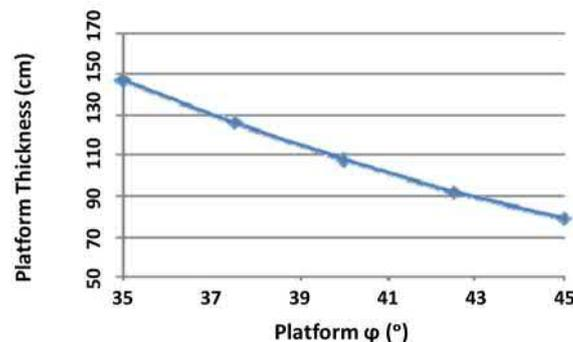
**Figure 14: Working platform thickness vs platform material internal friction angle (Batali et al., 2014a)**
