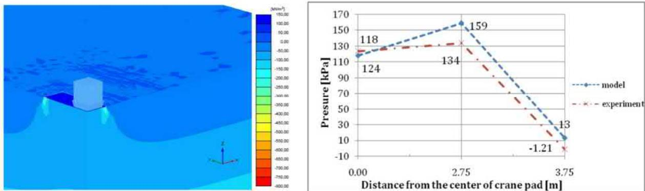
Figure 16: Numerical model results vs experimental measurements (Batali et al., 2014b)
