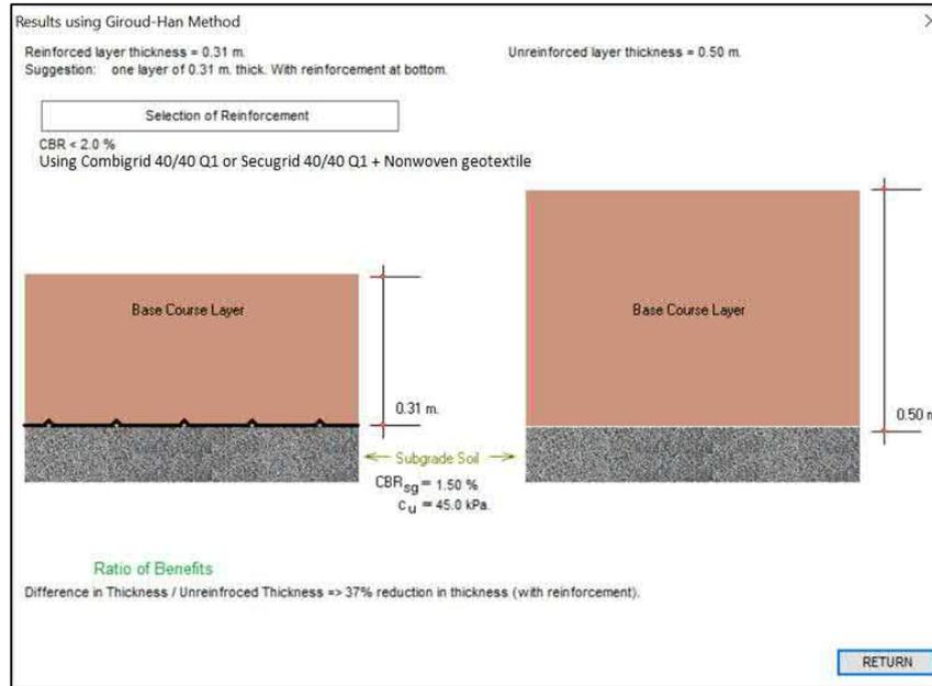
**Figure 7: Unpaved road design example using calibrated Giroud and Han (2004) equation for laid and welded biaxial geogrids**
