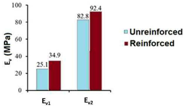
**Figure 10: Plate load test results for unreinforced and geogrid reinforced sections (Minazek and Mulabdic, 2014)**
