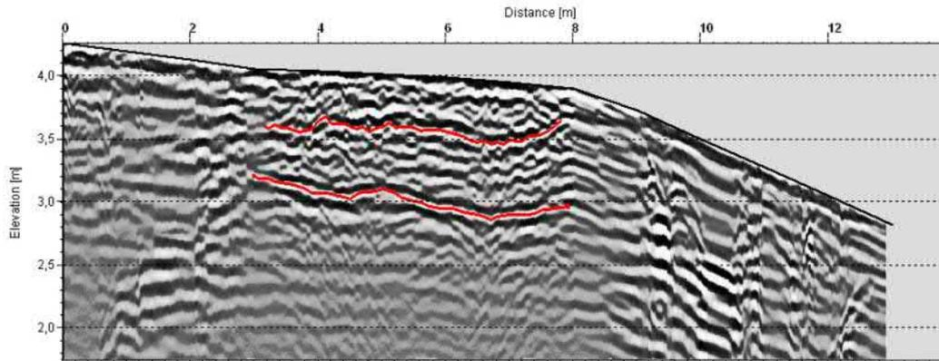
**Figure 2: GPR Survey Results, Geogrid reinforced floating road cross section (SNH, 2010)**
