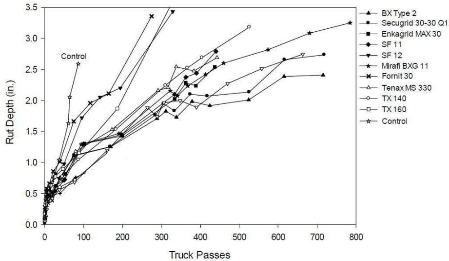
**Figure 6: rut depth results for sections stabilised with different geogrids (after Cuelho et al., 2014)**
