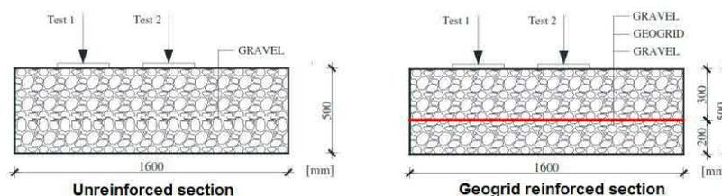
**Figure 9: Large-scale laboratory plate load testing (Minazek and Mulabdic, 2014)**
