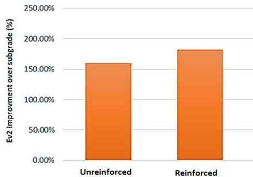
**Figure 11: Effect of geogrid reinforcement on  $E_{v2}$  improvement (after Shahkolahi et al., 2019)**
