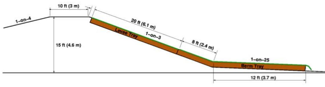
Figure 5 CSU test channel profile (Thornton et al., 2014)
