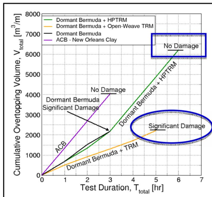
**Figure 7 CSU Wave Overtopping Simulator test results on non-reinforced vegetation, a HPTRM reinforced vegetation, an open weave TRM reinforced vegetation, and an Artificial Concrete Block (ACB) with clay subgrade (Thornton et al., 2014)**
