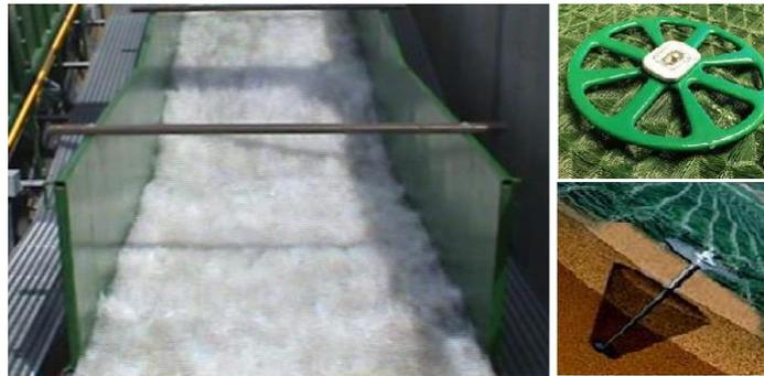
Figure 9 Wave Overtopping Simulator test Armormax® EEAS (Thornton et al., 2012)
