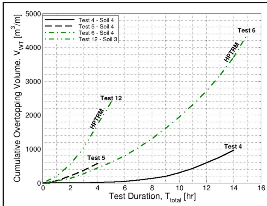
Figure 8 CSU Wave Overtopping Simulator test results on nonreinforced vegetation (test 4 & 5) and HPTRM reinforced vegetation (test 6 & 12) with sandy soil (Thornton et al., 2014)
