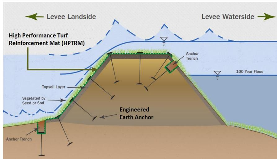
**Figure 2 Application of HPTRM Engineered Earth Armouring Solution (EEAS) in flood protection levees**
