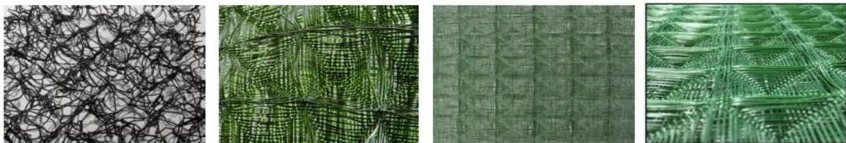
Figure 10 Different TRM and HPTRM products evaluated in the CSU wave overtopping test with different light penetrations of 90% (left), 35% (second from left), 25% (second from right), and 10% (right) (Thornton et al., 2018)
