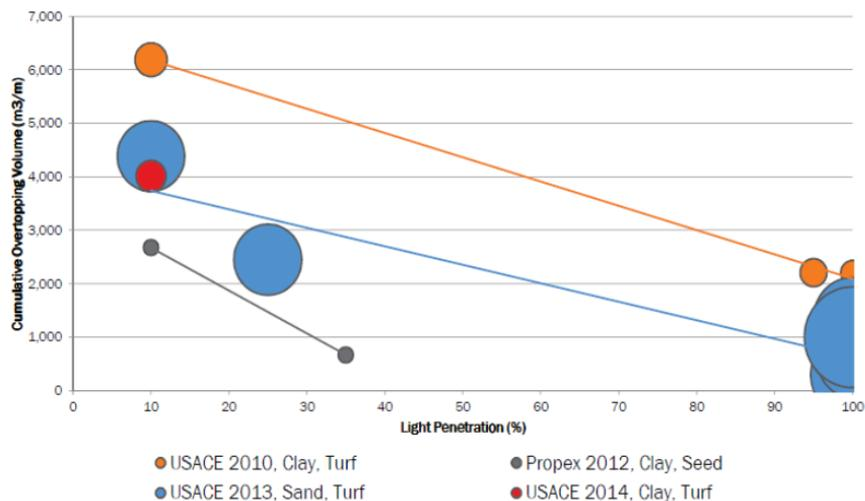
**Figure 11 CSU wave overtopping test results- Performance of TRMs/HPTRMs in terms of cumulative overtopping volume for different product light penetrations (Thornton et al., 2018)**
