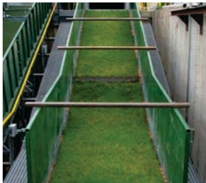
Figure 4 - ASTM D-6460 Test Plot
