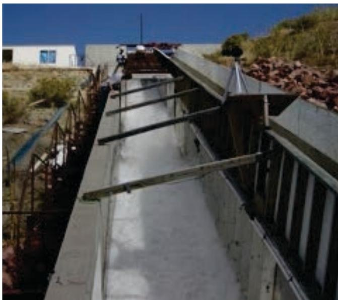
Figure 4 - ASTM D-6460 Test Plot
