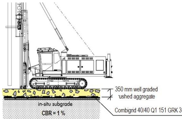
Fig. 3 Reinforced working platform
