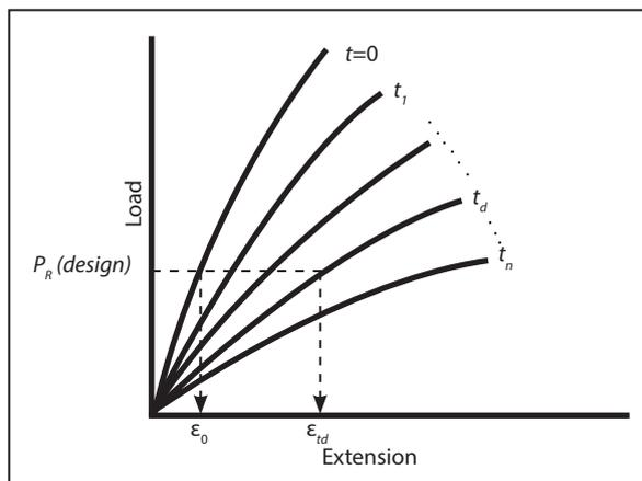
**Method of determining the initial extension  $\epsilon_0$  and the total extension  $\epsilon_{t,d}$  over time period  $t_d$  for geotextile reinforcement by use of isochronous creep curves**
