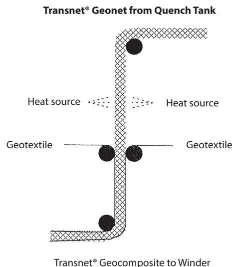
**Figure 1. Schematic of geonet-geotextile lamination process.**
