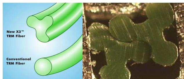
Figure 1. X3 fibres vs. round fibres
