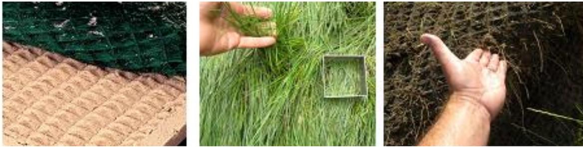
**Figure 2. Pyramid structure in TRMs (left), and the contribution with soil and vegetation in large scale hydraulic flume and field test (middle and right)**
