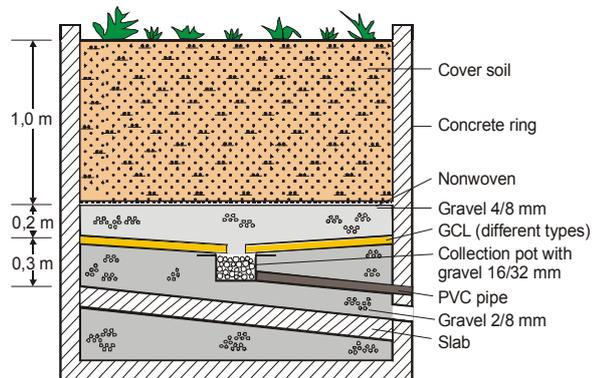
Figure 1. General layout of a lysimeter test set-up
