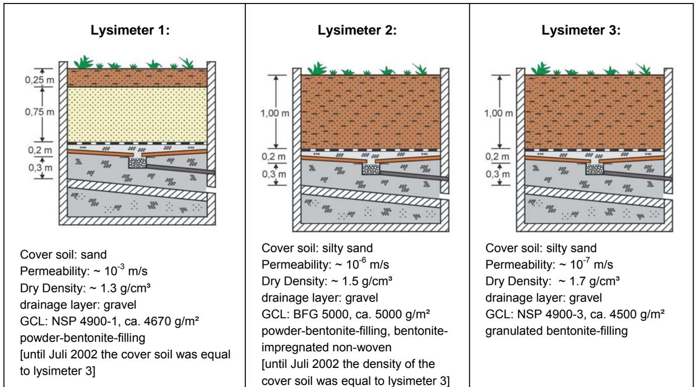
Figure 3. Lysimeter fillings
