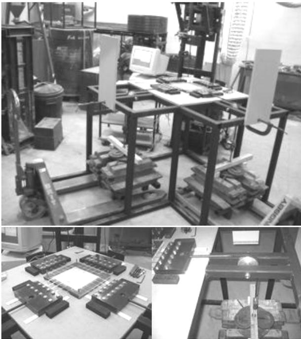
Figure 9 Biaxial Sustained Loading Test Apparatus
