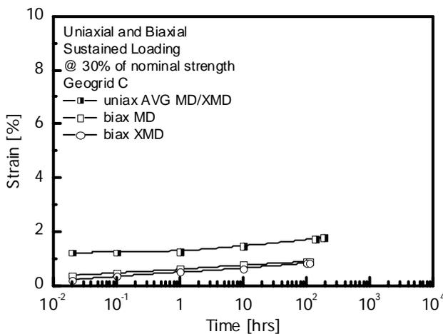
Figure 6 Uniaxial and Biaxial Sustained Loading Tests – Geogrid C
