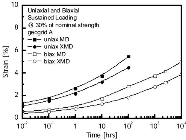
Figure 4 Uniaxial and Biaxial Sustained Loading Tests – Geogrid A
