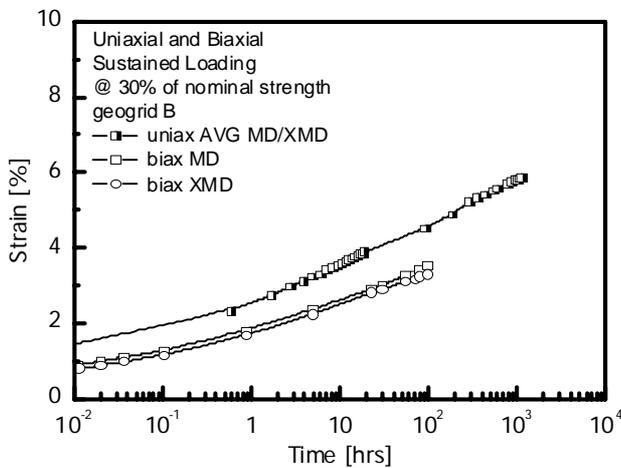
Figure 5 Uniaxial and Biaxial Sustained Loading Tests – Geogrid B
