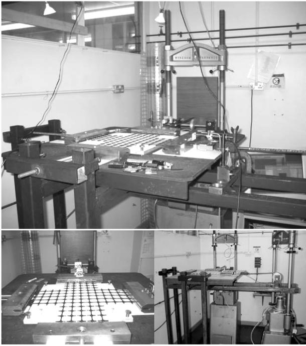
Figure 8 Biaxial CRS Test Apparatus
