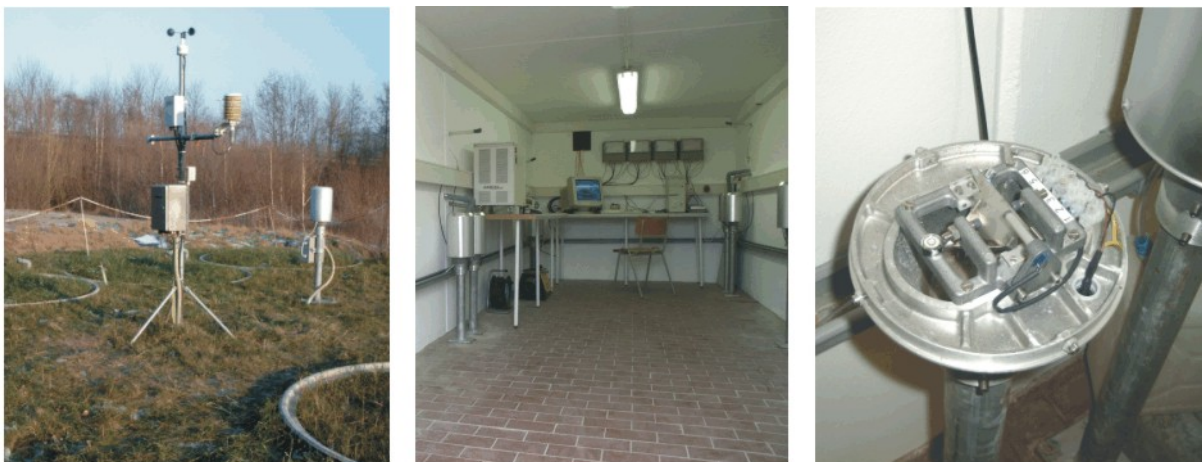
Figure 4. Meteorological station (left), measuring room (middle,) tipping bucket to measure water discharge (right)
