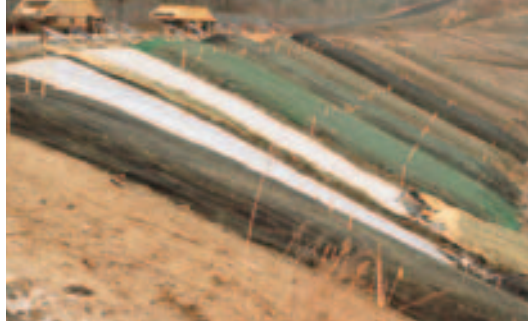
Figure 5 EPA field study on 2:1 slopes
