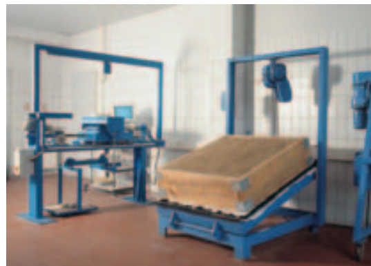
Figure 3 Automatic tilt-table and shear box
