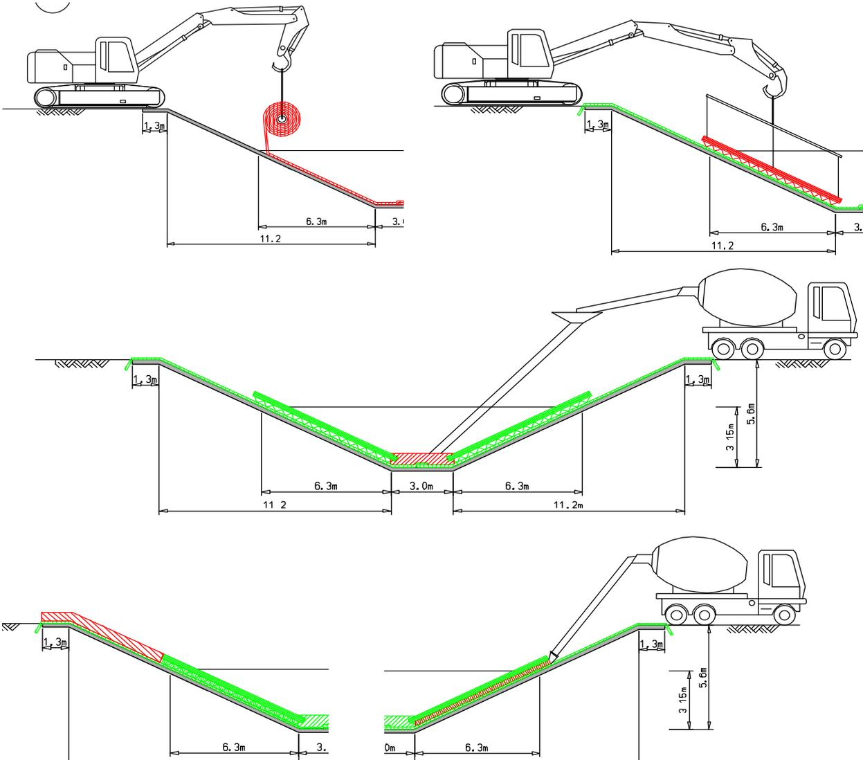
Figure 6: Underwater installation procedure with concrete slab facing (Ukraine, 2004)
