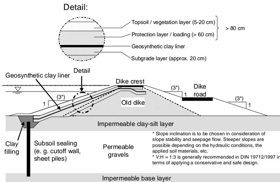
Figure 7: Application of a GCL in the course of dike refurbishment works (Haselsteiner & Strobl, 2006)
