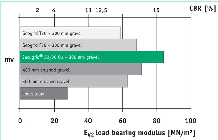
capacity results ( $E_{v2}$ ) with Secugrid®, averaged at 95.2 MN/m<sup>2</sup> (CBR: 14.5 - 19 %), ranging approximately 18.9 to 29.8 % higher than the other geogrid sections.
