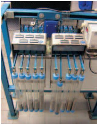
**Fig. 2:** Test device for Notched Constant Tensile Load Test (ASTM D 5397)
