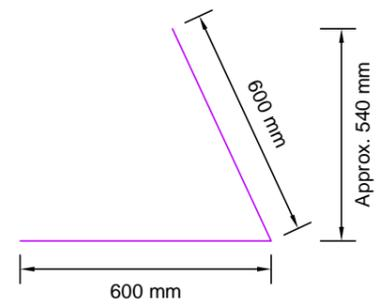
**Step 1** - Once the foundation has cut to its final level and compacted to meet the required bearing capacity, place the Terralink welded mesh facing on the level foundation. The Terralink panels are 2.4m long by 0.54m high (with an approximate tolerance of 3%) and is folded to a set facing angle of 65 degrees. Adjacent Terralink panels shall be overlapped by one mesh opening or a minimum 50mm. Alternatively the adjacent panels may be butted together and securely laced using hog rings.
